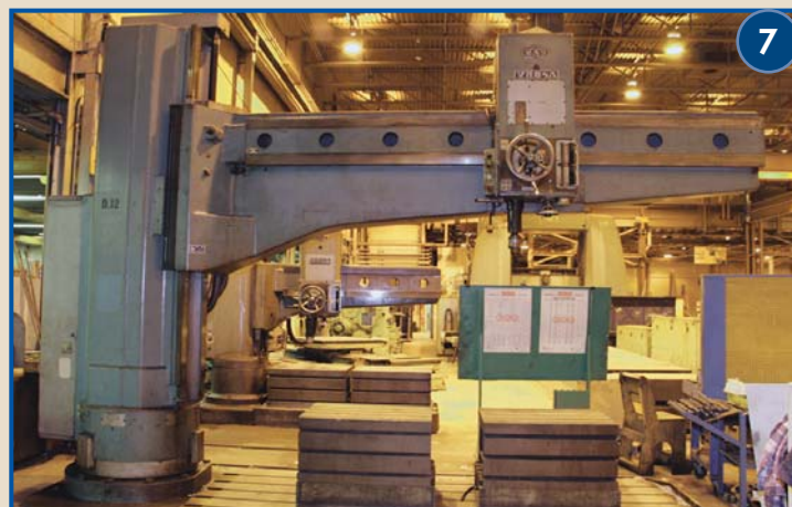
MAS 14' RADIAL DRILL MOD. VR84A
