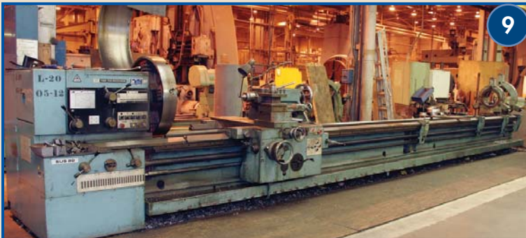
TOS SUS/8000 UNIVERSAL LATHE, 34" X 315"
