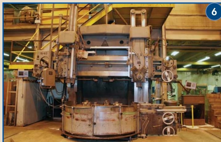
TOS SK16 63"/74.5" VERTICAL BORING MILL
